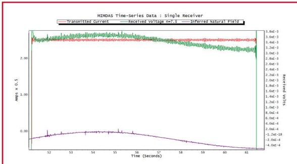
Figure 4: Blow-up of one on-period from the data presented in Figure 1. cursory analysis indicates that the received signal (green) is corrupted by irregularities in the transmitted waveform (red) and a lively natural electric field (purple). The MIMDAS system is unique in its correct treatment of both corrupting sources.
