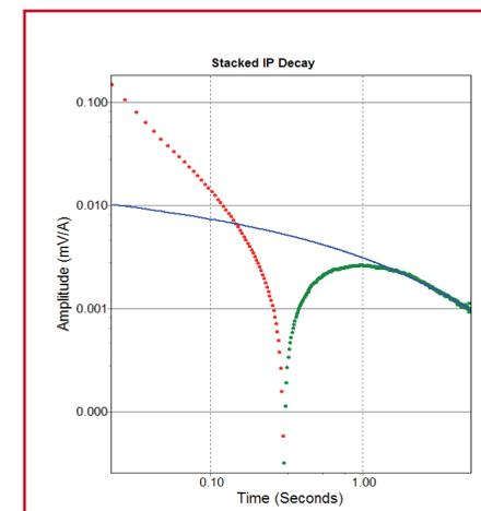
Figure 3: A Log-Log plot of the positive decay curve pictured in Figure 2. Negative EM Coupling (red) gives way to the polarisation decay past 0.2 seconds. A fitted Cole-Cole decay is plotted in blue to aid QC. Note that the positive portion of this clean decay is at a secondary voltage beyond some competitor's systems resolution!
