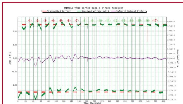
Figure 1: Time-series plot of 100% duty cycle transmitted waveform in Amperes (red), received Voltages at  $n=7.5$  (green) and calculated Inferred Natural Field (purple). Automatic selective stacking has rejected the cycles in red from the stacking process.
