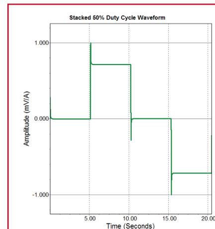
Figure 2: The stacked system response derived from the data in Figure 1, convolved with a unit 50% duty cycle frequency response, plotted in the time domain for easy QC.
